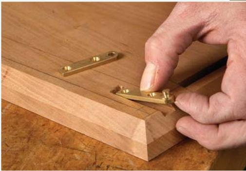
**4 Set the hinge in place.** The hinge leaf should be flush to the surface of the workpiece. Drill pilot holes before attaching it with screws.
