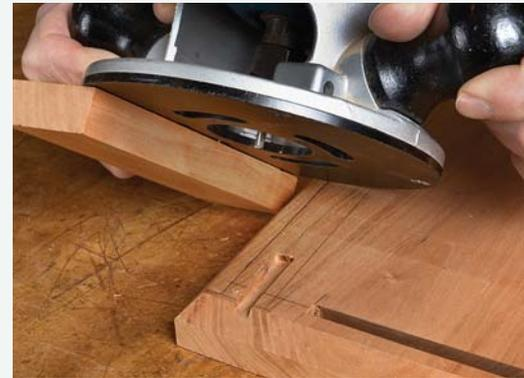
**3 Rout it out.** Hog out the waste in the mortise using a small straight bit. Position the edge guide so it makes a clean cut along the rear edge of the mortise.
