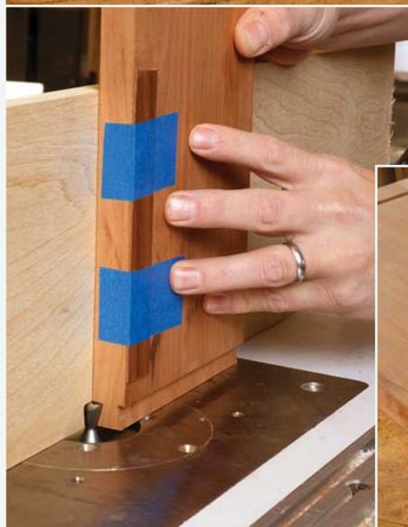
**2** *Cut a tapered tail.* With the same dovetail bit partially buried in the fence, cut a tapered tail by attaching the same shim material to the rear outer edge of the side stock.
