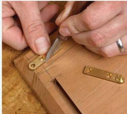
**2 Score around the hinge.** Use double-sided tape to hold the hinge in place and then scribe its location with a marking knife.
