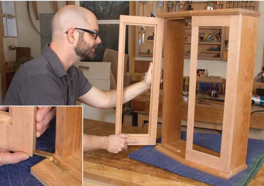
**6 Hang the door.** Attach the hinge leaves to the cabinet and one side of the door. Set the leaf attached to the door in place on the hinge. Set the other leaf in place on its hinge and slide the door into place. Double-check the position of the door on the case and then mark out the screw holes. Finish the doors and install the glass before you attach the doors permanently.
