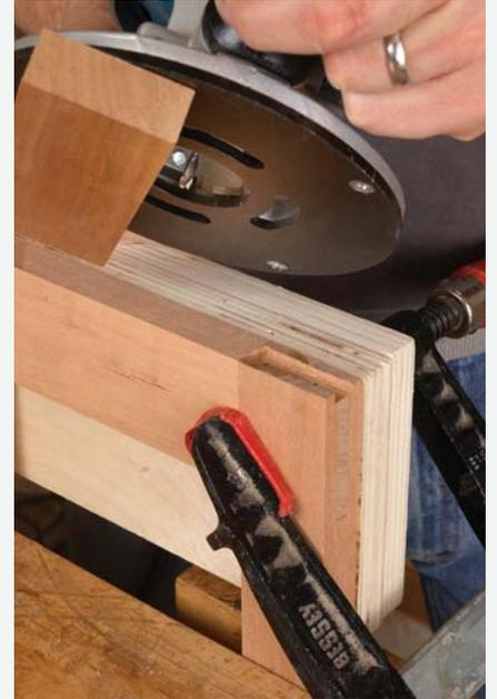
**5 Rout the door mortise.** Scrap stock clamped flush to the top of the door allows you to rout the door mortises in the same fashion as those on the case.
