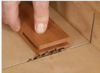
**2** **Cut tenon shoulders.** Set the blade to match the thickness of the mortise walls. Then use a stop-block on a table saw sled to cut the tenon shoulder.
