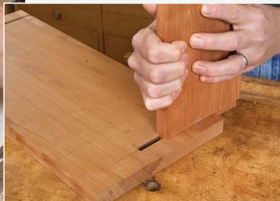
**3** *Test the fit.* Remove stock from the tail stock gradually, testing the fit until it slides snugly into the slot.
