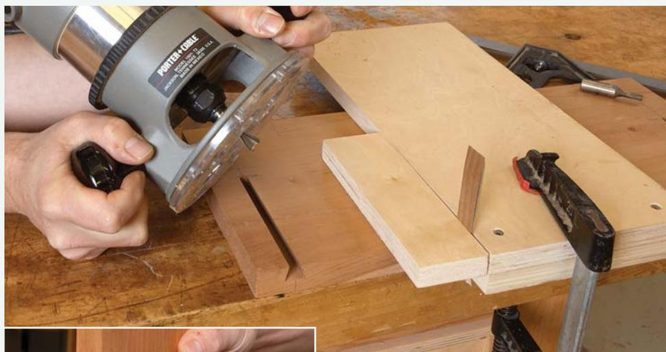
**1** *Take two passes.* Cut a tapered dovetail slot by shimming out the leading edge of the guide fence and recutting the dovetail slot.
