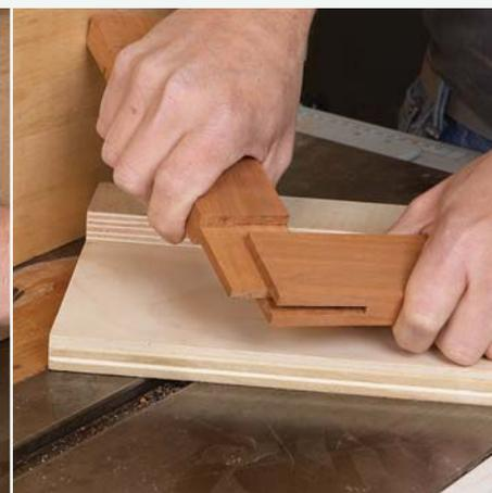
**4** **A snug fit.** Aim for a tenon that slides into the mortise with a little resistance using only hand pressure.
