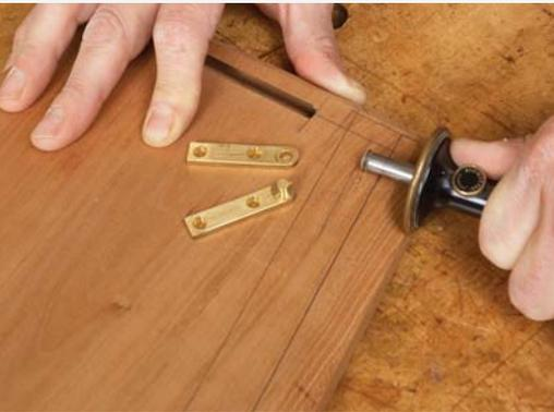
**1 Positioning the hinge.** Draw out the position of the door stock to help center the hinge. Then use a marking gauge to establish the front and rear edges of the hinge mortise.
